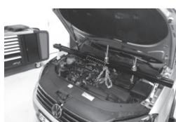
Fasten the engine using one or both pairs of adjustable hooks.
