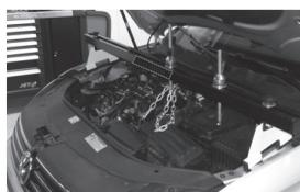
Fit the engine support. Place the pads on a strong zone on both sides of the vehicle.
