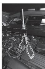
Use the fastening eyes included to handle the engine.
